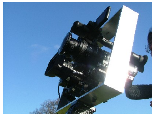
Camera Rig with standard and fisheye cameras
